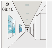
When the natural light level exceeds setpoint off to light, the light will turn off even if when the space is occupied.
