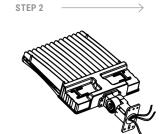
Install the attachments and tighten the screws according to the blown up photo.
