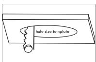
Use the 6" hole size template in the packaging to cut a hole on the ceiling for installation.
