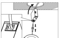
Connect downlight to junction box. Select your favorite color temperature by using the 5CCT switch on the junction box. Place junction box into the ceiling.
