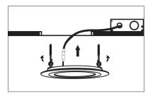
Push the easy mount clips up and insert the downlight into the ceiling, release clips to mount the downlight on the ceiling.
